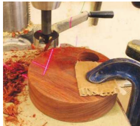
▲ Pic.12 Clamp the block to the drill table. The laser on his Jet drill press is fantastic when you are lining up where to drill. Drill slowly so you don't burn the timber
